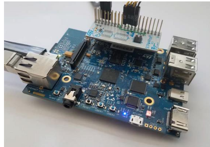
Example of SECURE infrastructure implementation using STM secure elements STM32 and TPM with Linux
